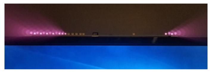
The Regular setting works best with Screen Sizes 10 inches, up to 40 inches (and possibly larger, why not give it a try). When you set it to Regular, the inner LEDs are turned on. The illumination isn't as high with the Regular setting, because you will be using the guns closer to the screen, so the illumination doesn't need to be as high. Also, with the Regular setting, the LEDs are closer together. This allows you to use your guns closer to the screen then you otherwise could:
