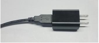
USB ports typically supply volages in the range of 4.75v to 5.25v. This sensor bar can handle these voltage ranges without any issues. The LEDs that we use on this sensor bar are very high quality and could even handle higher voltages then this, but it's not advised. Suppying more power produces more heat, and it doesn't improved your light gun's tracking when applying more voltage.
