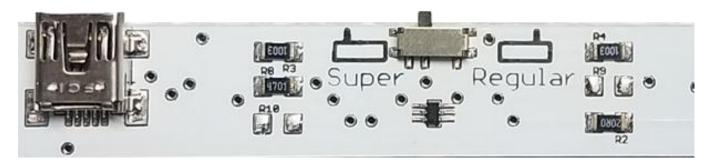
The Super setting works best with Screen Sizes 32 inches, up to 100 inches (and possibly larger, but this can depend on a lot of factors. We only officially support screen sizes up to 100 inches with this sensor bar). As you can see, the outer LEDs are turned on when the switch is set to Super. The illumination is higher with the Super setting. Having higher illumination enables support for greater distances from the screen:
